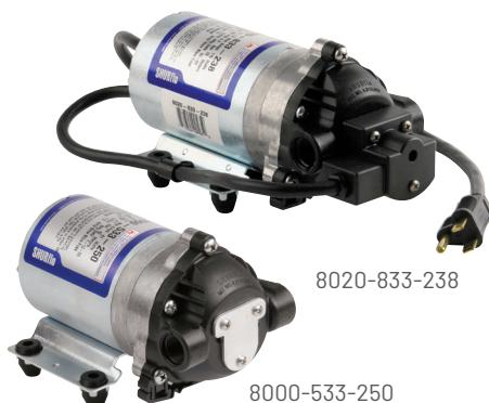
These Shurflo 8000, 8090 and 8020 Series bypass and demand pumps provide the same reliability as the 12 VDC version, except in a 115 VAC or 230 VAC capacity. They are ideal in agricultural applications that require high pressure with flow rates up to 1.6 GPM [6.1 L/min] and low amp draw. They can be mounted in any position, are compact, and are designed for easy maintenance.
