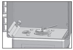
Final assembly is as shown. If all positions in cord seal are not used, fill open positions with PVC plugs provided. Tighten the nut on the cord seal to prevent gas and moisture from entering panel.
