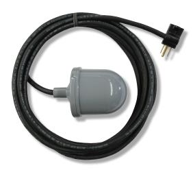
The Mini Doser™ Pump Switch is used to turn a pump on and off in environments with temperatures up to 140° F. This product can be used for a variety of applications, including but not limited to: septic tanks, sump pits, holding tanks, pump chambers, water tanks, and any other liquid tanks. Available in 120/230VAC bare lead (no plug), 120VAC piggyback plug, and 230VAC piggyback plug, 15 Amp models.
