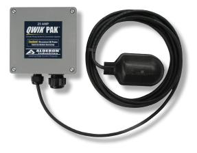
The Qwik Pak<sup>™</sup> High Amp Pump Switch (25 Amp) is typically used to operate a high amp pump using a control float switch and control relay. The enclosure serves as a junction box with the pump and incoming power wires terminated with the included Wago quick connections.
