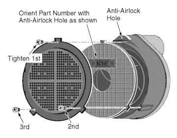
Assemble Screen and Shield as shown.
