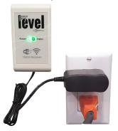
Remove the lid on the transmitter and insert the provided AA batteries into the transmitter. You should see the status LED blink three times slowly to indicate a successful connection with the receiver
