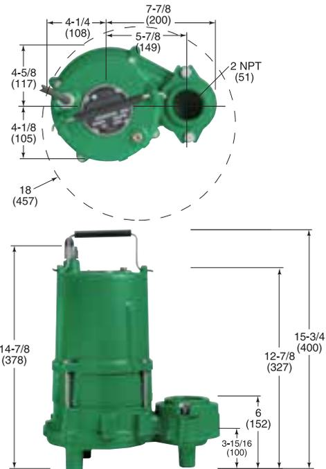
All dimensions in inches. Metric for international use. Component dimensions may vary  $\pm 1/8$  inch. Dimensional data not for construction purpose unless certified. Dimensions and weights are approximate. On/Off level adjustable.
