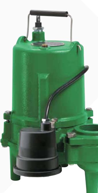
The Hydromatic SP50 submersible pump is specifically designed to meet the demands of handling wastewater and sewage in residential and commercial building applications. The 2 inch NPT discharge pump (3 inch discharge optional) is available with a powerful 1/2 horsepower motor, in both automatic and manual configurations; and can handle capacities up to 150 gallons per minute and heads to 29 feet.
