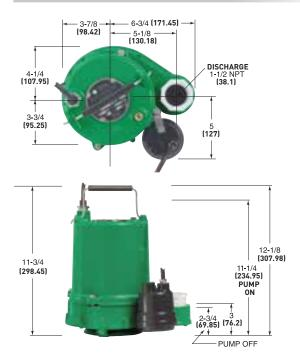
All dimensions in inches. Metric for international use. Component dimensions may vary  $\pm$  1/8 inch. Dimensional data not for construction purpose unless certified. Dimensions and weights are approximate. On/Off level adjustable.
